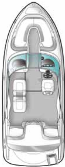
Standard Seating Plan Bow Rider w/Removable Cushions & Storage Below; Helm Bucket Seat w/Sport Logo & Swivel & Slide Functions; Hi-Lo Aft Jump Seats w/Motorbox; Port Back-to-Back Lounger
